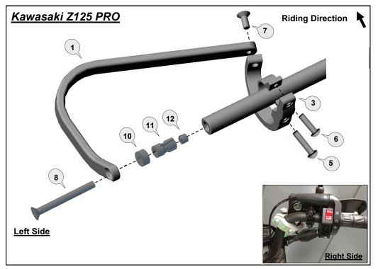
**<u>FITTING TIP</u>:** *Kawasaki Z125 PRO* Clamp is positioned below the bend of the handlebar as shown.
