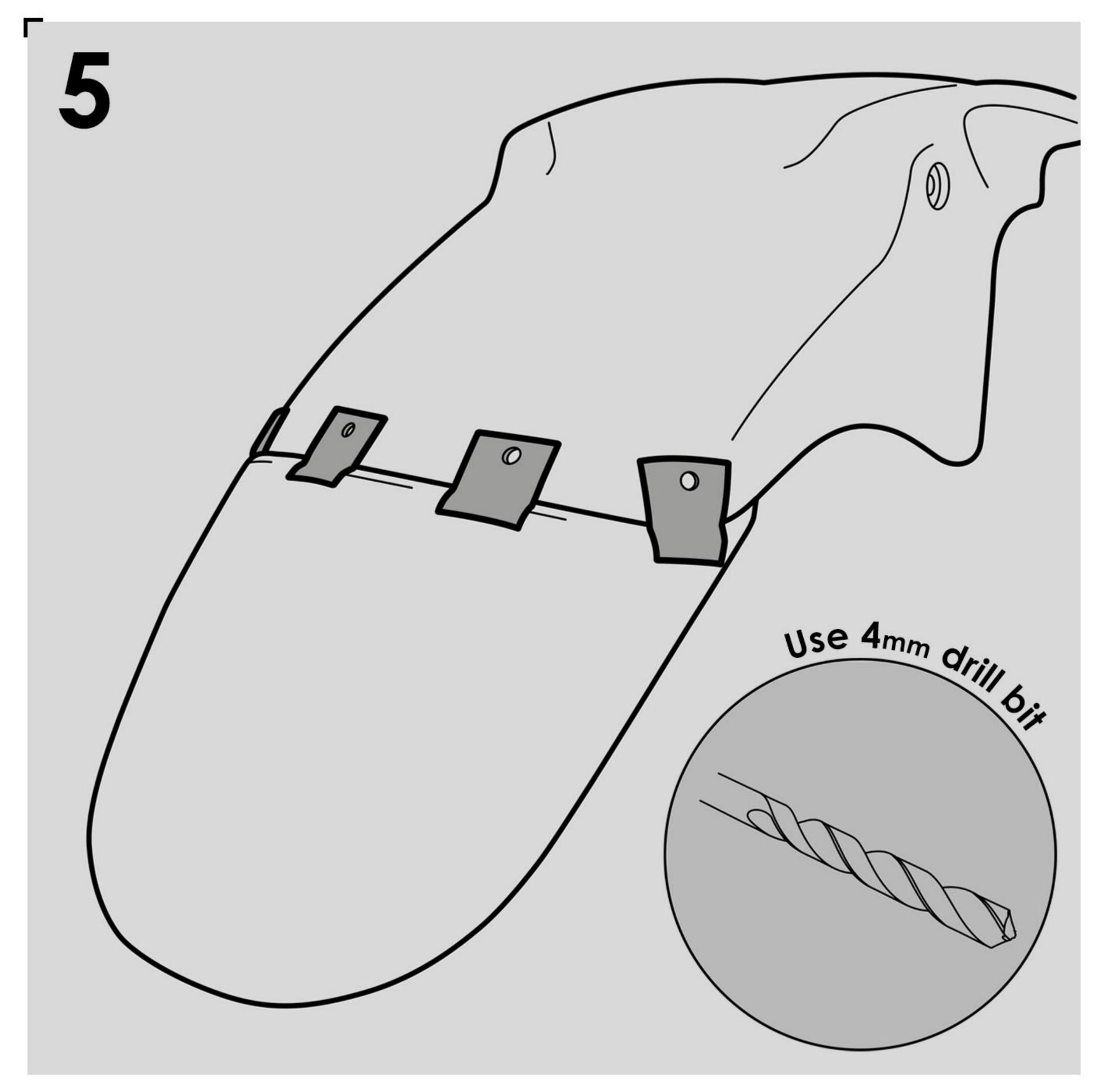
Use masking tape to mark equally spaced drilling points.
