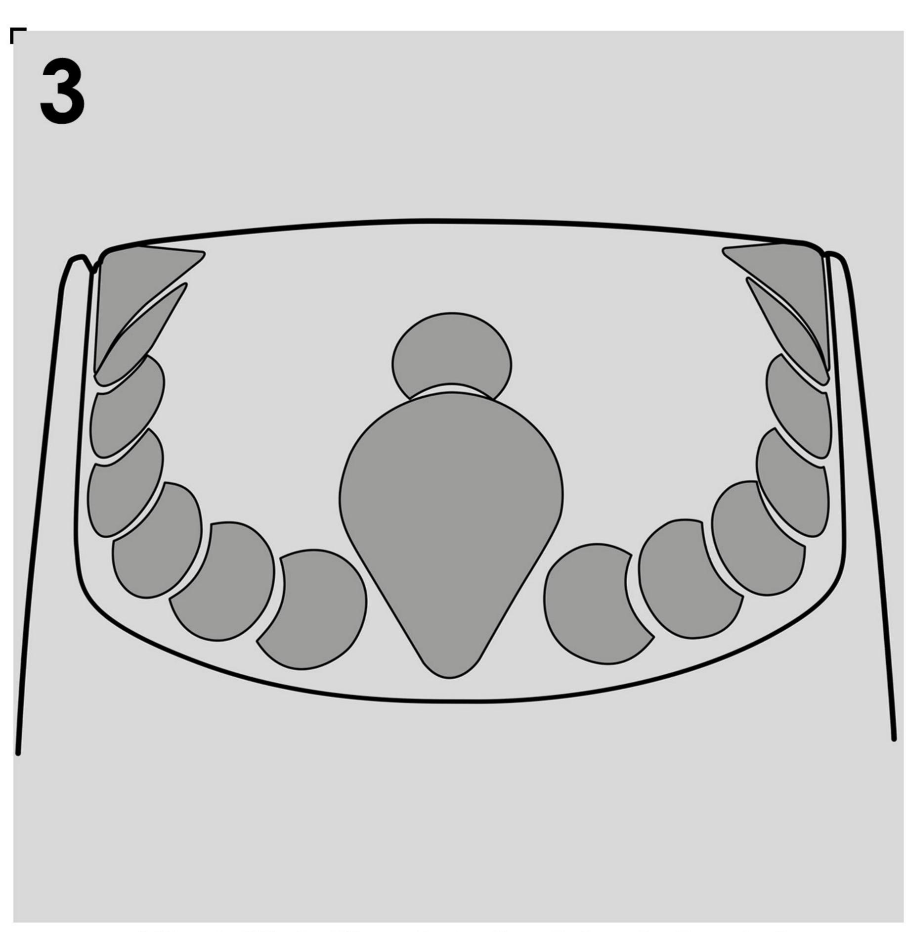
Attach Stick-Fit pads to the Extenda Fenda/ Hugger Extension using this diagram as a guide. Avoid recesses & corners in the moulding as this will effect the fit.
