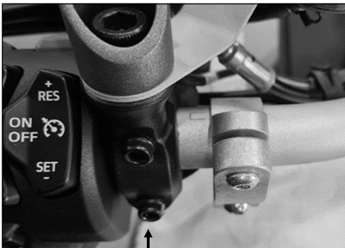
(Appropriate setup shown of the clutch lever housing when repositioned)
