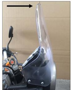
For Maximum Clearance With the four screws loose, gently push forward at the top of the
