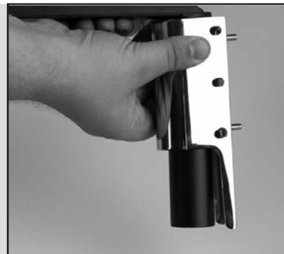
Figure 9. Rotate studs to outside.
