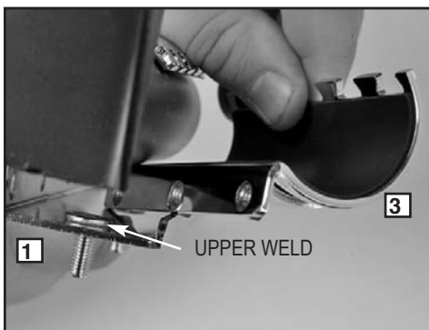
Figure 10. Hold Outer Bracket (1) LOW on Triple Clamp. Inner Bracket (3) must slide between UPPER and LOWER WELD STUDS.
