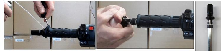
**TIPS:** To help with applying lubrication to the inside of the handlebar, loosen throttle housing and slide inwards. For left side use a screwdriver to lever grip end away from handlebar end. Be careful not to get lubrication between grip and outside of handlebar.
