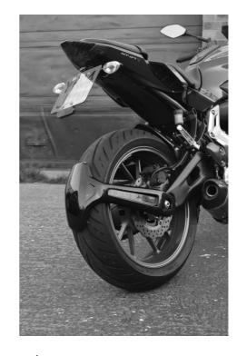
Check all positions for clearance before your first ride. Bear in mind that there will be some movement of the Spray Guard head whilst riding. Also check that clearance is maintained after your first ride. It is important that this Spray Guard remains rigidly mounted at all times. If it is allowed to loosen permanent damage will be caused to the moulded castellation on the reverse of the Spray Guard.
