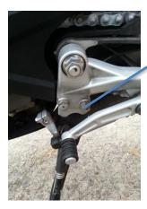
1. Remove the bolt on the bottom right of the gear pedal assembly and loosen (not remove) the ones on the bottom right and centre
