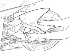
**4** Secure the hugger in place using the Three original fixing points and bolts removed in step **1**.
