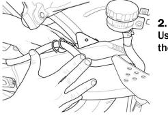
Using the original bolt, secure the mounting bracket **between** the brake line holder and the swinging arm.
