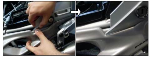
4. Firmly push the Infill Panel Locking Clip under the Rear Seat leading edge. Press both parts together and slide the Infill Panel underneath.
