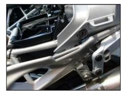
3. Slide the panel up and over the left pannier mounting bracket. Slide the frame mounting grip (with foam) up and clip into position.
