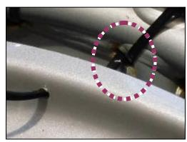
5. Thread the cable tie through the hole in the Infill Panel. There is a hole in the chassis frame where other cable ties are present that is lined up with the hole in the Infill Panel. Thread the cable tie through the chassis and tie up tight. Cut off any excess as necessary.
