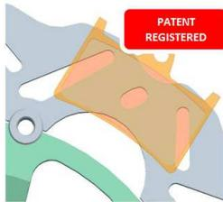
Outer and inner diameter of the disk have a non-round design that enables better radial expansion of the rotor under extreme heat conditions. Moreover piercing holes are replaced by edges specifically designed to grow brake pad regeneration process
