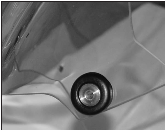
Figure 4 Showing Exterior Bushing
