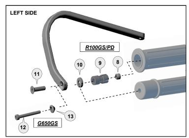
Loosely assemble clamp to the handlebar with applicable parts. Attach the handquard backbone with applicable parts to the handlebar end and also to the clamp connector (7).
