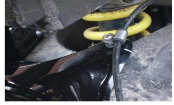
Next fit the rear mounting point on the exhaust can side with the brake hose clip on top of the
