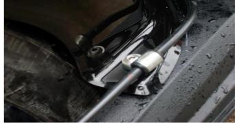
Now fit both mounting points on the chain guard side and tighten all mounting points fully. Finally re-fit the exhaust can.
