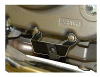
Remove the two <u>rearmost</u> (of three) 8mm sump bolts directly under the crank case on the <u>left hand</u> side of the bike and fit bracket supplied marked "B" with same bolts and with stepped section facing outwards. Make sure to tighten bolts.
