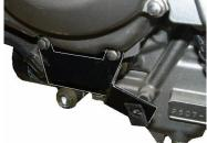
Remove both 10mm bolts securing top of oil radiator to fixing bracket on bike (one each side top of exhaust) and insert supplied big bracket marked "A" facing forward from behind oil rad to line up all holes, trapping new bracket between original bracket behind, and existing rubber washers in front. When all is lined up and new bracket is seated upright behind oil rad replace both 10mm bolts and tighten.
