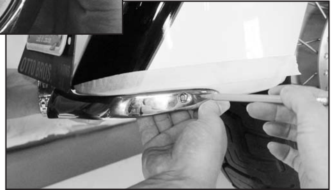
Figure 1. Tape Fender, Position Fender Tip, Mark Fender
