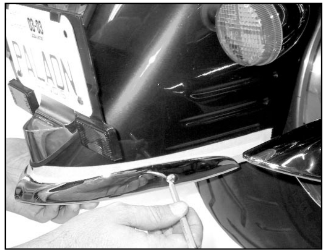
Figure 1. Tape Fender, Position Fender Tip, Mark Fender
