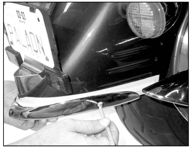
Figure 1. Tape Fender, Position Fender Tip, Mark Fender
